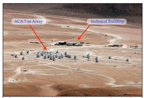
Figure 6: An areal view of ALMA in a relatively compact configuration. The maximum distance between the 12-m Array antennas in the most compact configuration is less than 200 m, and the minimum distance a mere 15 m. Indicated also are the AOS Technical Building, and the ACA 7-m Array. (Credit: C. Padilla/ALMA (ESO/NAOJ/NRAO))
