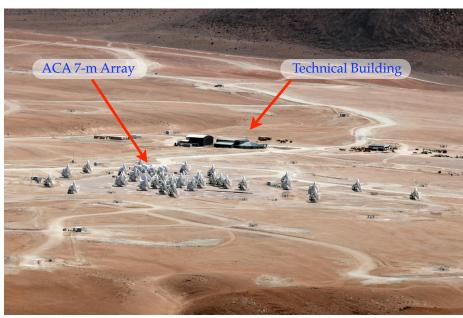
Figure 6: An areal view of ALMA in a relatively compact configuration. The maximum distance between the 12-m Array antennas in the most compact configuration is less than 200 m, and are as close together as 15 m. Indicated also are the AOS Technical Building, and the ACA 7-m Array (Credit: C. Padilla/ALMA (ESO/NAOJ/NRAO))
