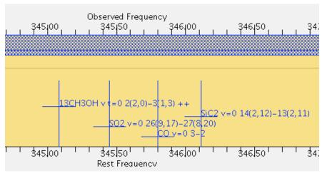
Figure 36: Four spectral windows were set up to observe these four lines simultaneously in one baseband using the OT. The windows are each 234 MHz wide (with 0.43 km/s channels), and are centered at 345.80, 345.45, 346.11 and 345.09 GHz. The spectral windows must fit within the 2 GHz wide baseband.
