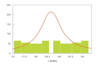
After the signals enter the horn they are down-converted to lower frequencies and divided into four channels on either side of the emission line. This is illustrated in Figure 7.
