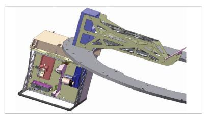
Figure 5. Drawing of the Relay and Radiometer. (Courtesy of Omnisys Instruments AB)
