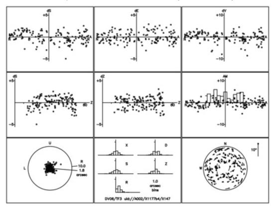
Here is the analysis (made with the TPOINT<sup>™</sup> package from Patrick Wallace) of such an interferometric pointing run demonstrating conformance with the ALMA requirement of 2 arc second rms accuracy over the whole sky.
