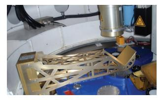
Figure 3. The Optical Relay which takes the signal to the Water Vapour Radiometer.
