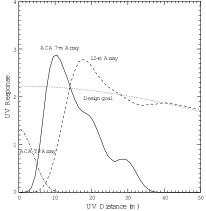
Fig. 2. This shows the response of the ALMA instrument to sources of extended emission. There are three components: the 12m Array which consists of the antennas in the interferometer array (response is shown as a dashed line), the four 12 m antennas used for total power measurements in the ACA TP Array (response is shown as a dashdotted line), and the twelve 7m antennas (response is shown as a solid line).
