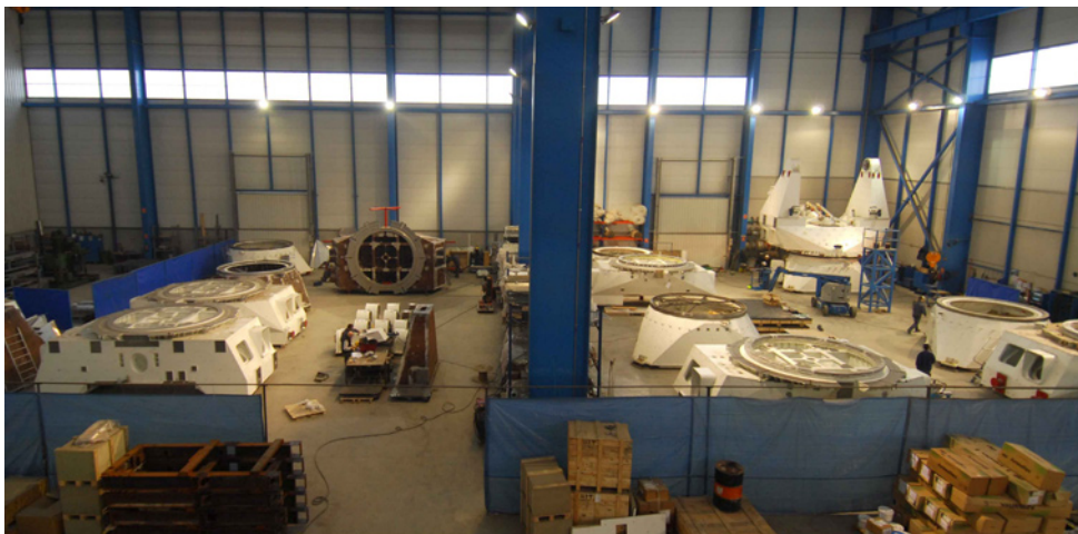
The production of the antennas is spread among various countries. In this photo, the Asturfeito facilities in northern Spain where the steel structures of the European antennas are being built. Shown are the AEM antenna bases and yokes in different phases of assembly.
