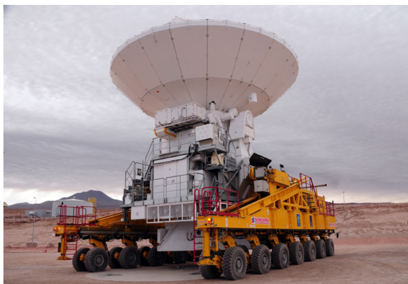
In this picture, the antenna has just been lifted from its foundation at the OSF. From then, will start the move of the antenna to its final destination at 5000 meters.
