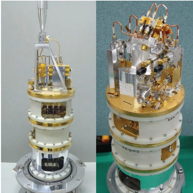
Two different ALMA Front Ends. Band 4 (on the left) operates from 125 to 163 GHz and is designed and built by NAOJ in Japan. Band 8 (on the right), also built by NAOJ, is designed to operate at much higher frequencies (385 to 500 GHz), which reflects in the different design.
