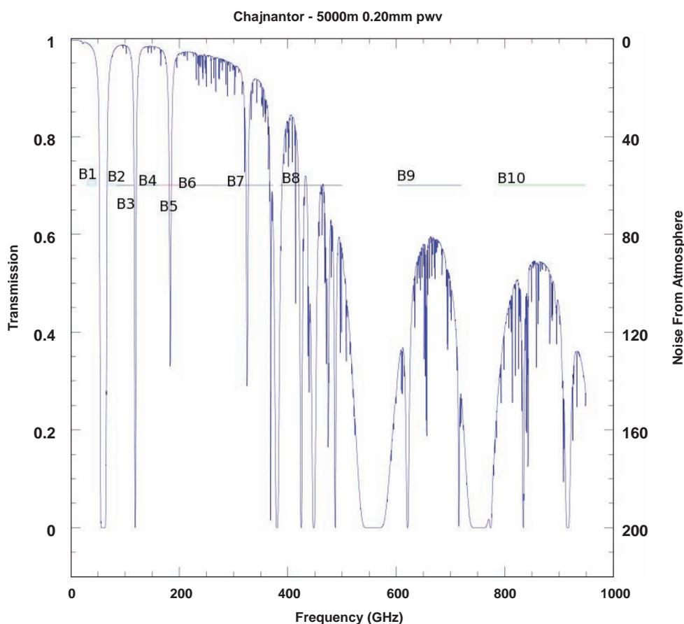
*On the left vertical axis is the transmission of the earth's atmosphere, on the right axis is the noise contributed by the earth's atmosphere. This plot is for the ALMA site, at an elevation of 5 km. The total amount of water vapor above the site is 0.25 mm. This is a very small amount of water vapor, so the effect of the earth's atmosphere on receiver noise is a minimum.*
