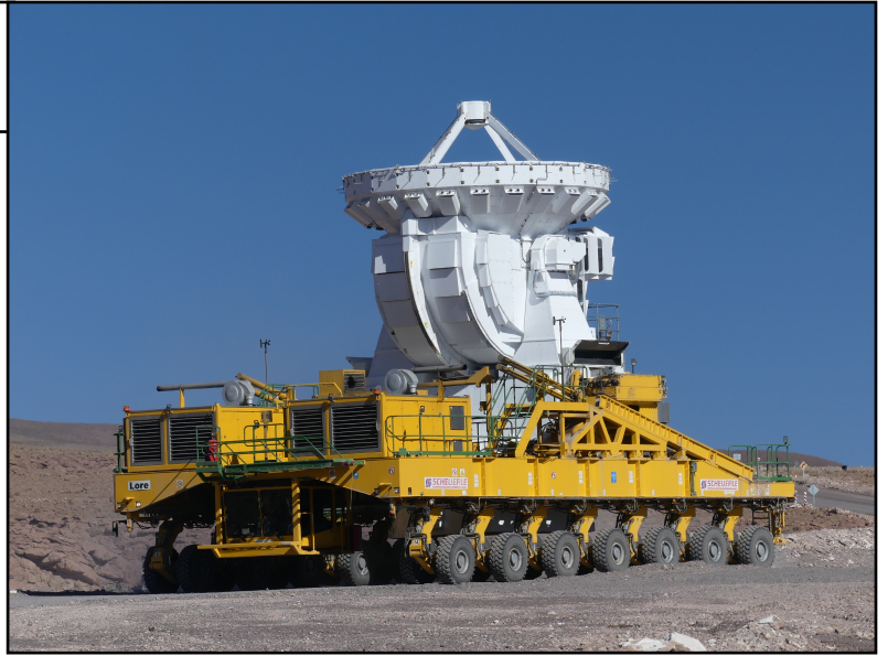
Figure 35: The ALMA transporter carrying one of the 7-m Array antennas to the OSF for servicing. (Credit G. Schieven)
