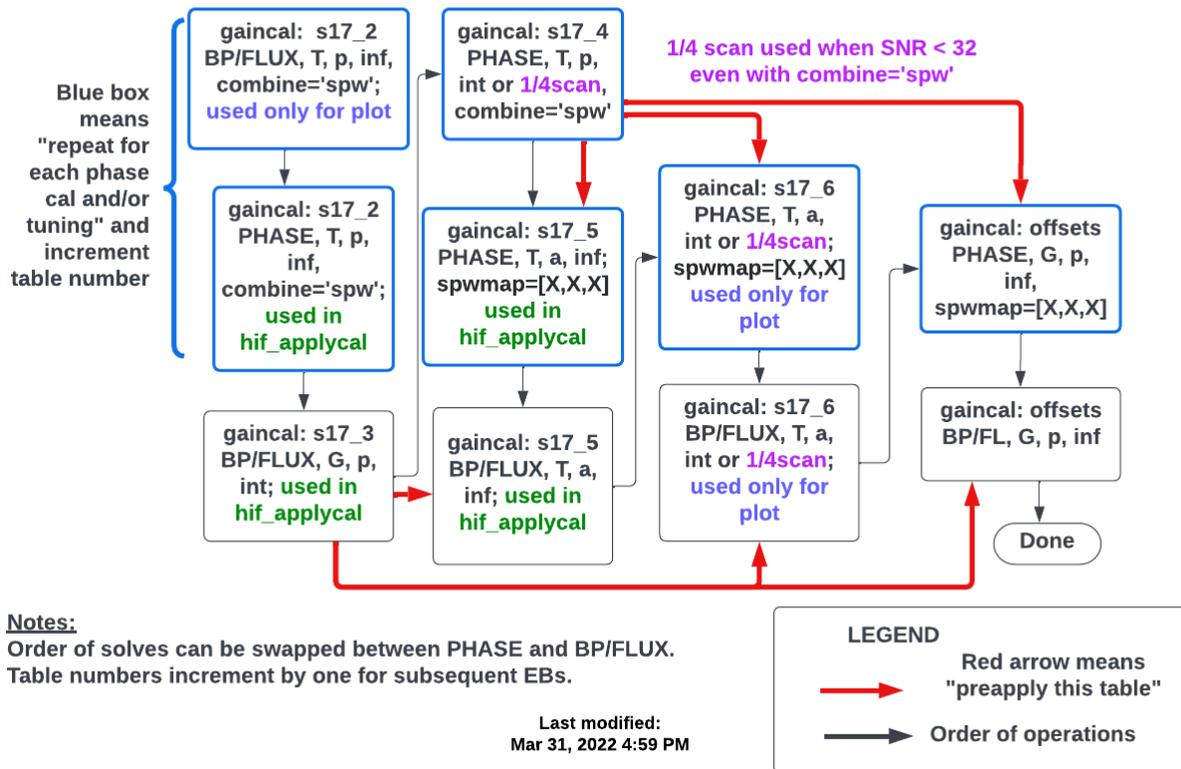
Figure 32: Logical flow in hifa\_timegaincal for the case of low SNR in all spws.
