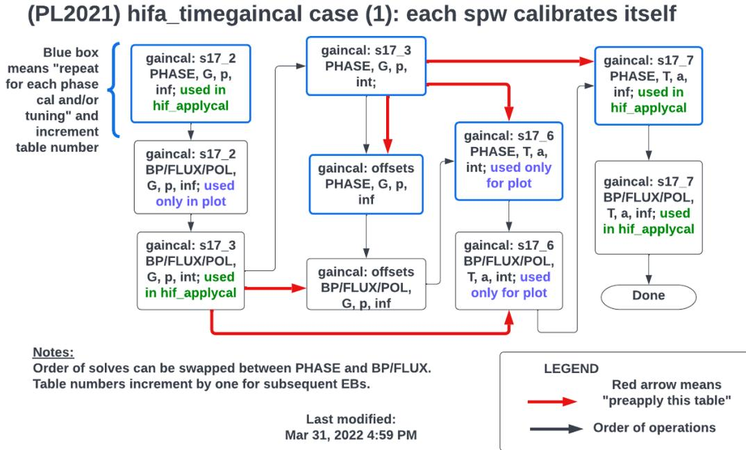
Figure 60: Logic flowchart of `hifa_timegaincal` for the case of high SNR in all spws in PL2021.
