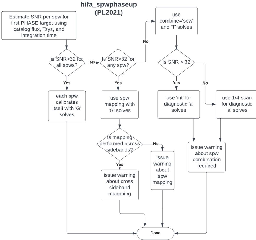
Figure 56: Logic flowchart of `hifa_spwphaseup` for determining the temporal gain strategy in PL2021. Compare to the PL2022 version in Figure 23.
