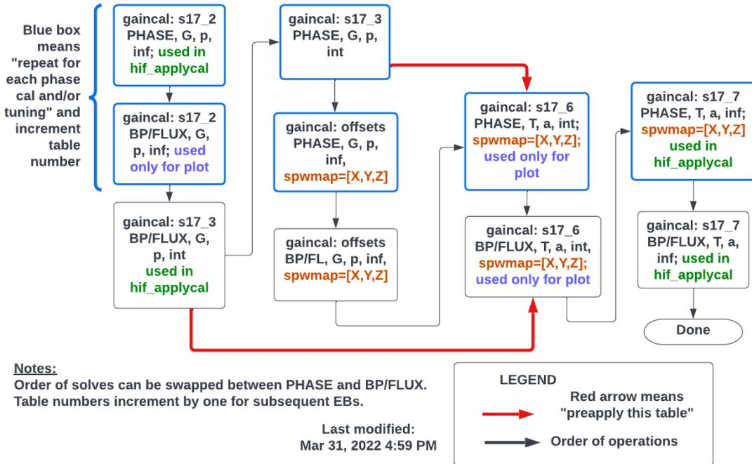
Figure 61: Logic flowchart of `hifa_timegaincal` for the case of high SNR in at least one spw (but not all spws) in PL2021.
