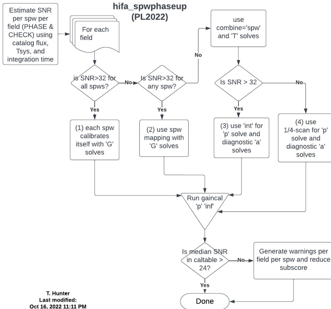
Figure 23: Logic flowchart of `hifa_spwphaseup` for determining the temporal gain strategy. Compare to the PL2021 version in Figure 56.
