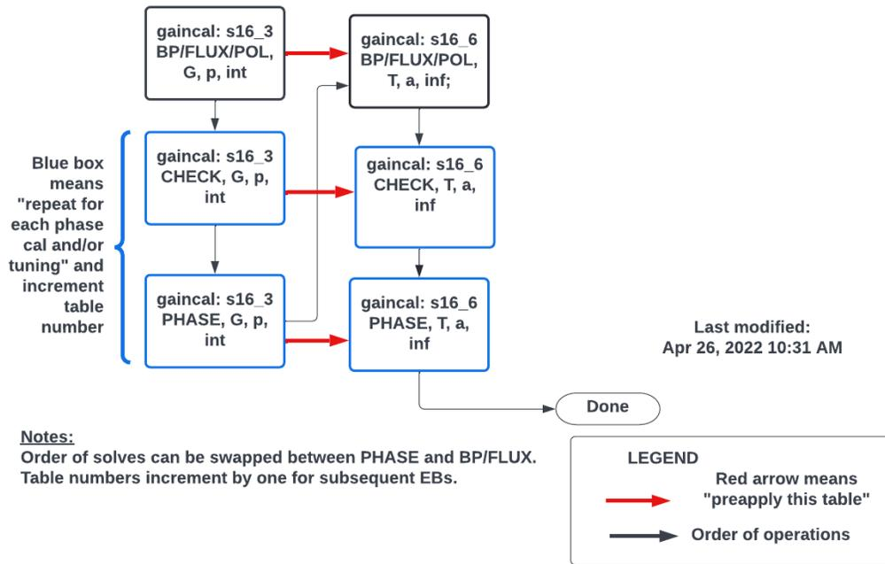
Figure 57: Logic flowchart of `hifa_gfluxscale` for the case of high SNR in all spws in PL2021.
