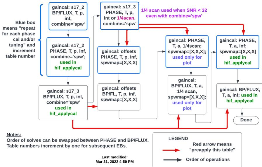
Figure 62: Logic flowchart of `hifa_timegaincal` for the case of low SNR in all spws in PL2021.
