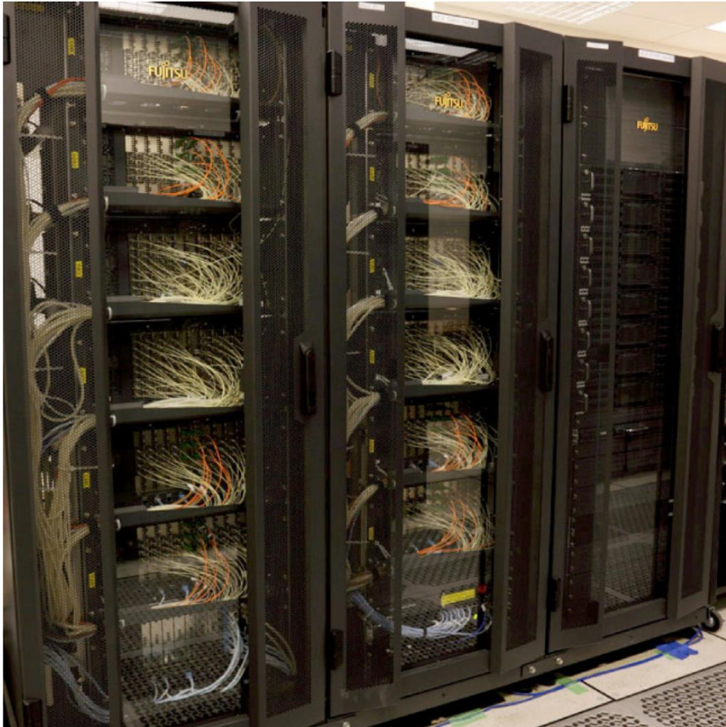
Figure 5.4: Two quadrants of the ALMA Compact Array (ACA) correlator installed in the ACA correlator room. Credit : ALMA (ESO/NAOJ/NRAO), S. Okumura
