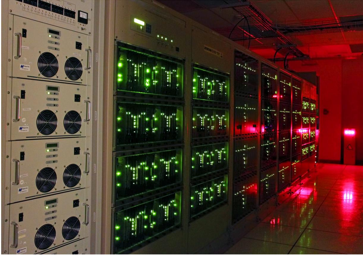
Figure 5.2: The ALMA 64-input Correlator. This view shows lights glowing on some of the racks of the correlator in the ALMA Array Operations Site Technical Building and shows one of four quadrants of the correlator. Credit: ALMA (ESO/NAOJ/NRAO), S. Argandoña
