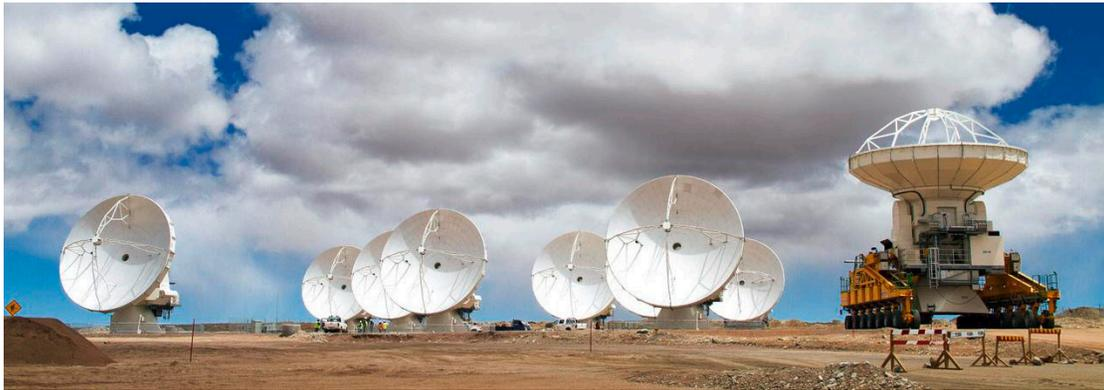
Figure 3: Another ALMA antenna takes its place at Chajnantor, carried by one of the two ALMA transporter vehicles. (Photo J. Guarda, © ALMA (ESO/NAOJ/NRAO))
