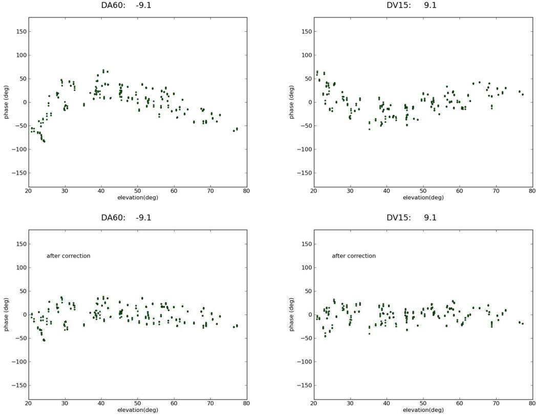
Figure 1: **Top Row:** The residual phase versus elevation for the two antennas, DA60 on A090 and DV15 on A089, with the maximum height difference in configuration C32-5. Each point represents the phase residual for a 20-sec scan, after removing the best baseline parameters for the antenna. **Bottom Row:** shows the residual phase versus elevation after correcting the phase for the delay associated with the antenna height difference.. The elevation dependence is largely removed.
