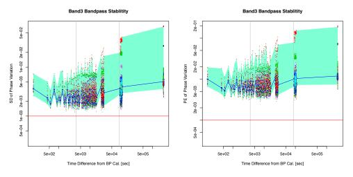
Figure 4: Band-3 bandpass variation. Small colored dots stand for antennas and polarizations. The mint filled area indicates the range of dots and the blue circles with solid lines indicate the median values. Two gray vertical lines point the timescales of 1 hour and 1 day, respectively. The red horizontal line indicates the required stability of  $-30~\mathrm{dB}$ .
