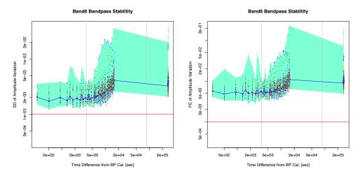
(a) SD (left) and PE (right) of bandpass amplitude variation at band 6.
