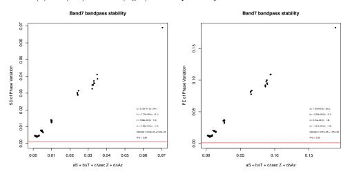
Figure 25: Predicted and measured bandpass variations in Band 7
