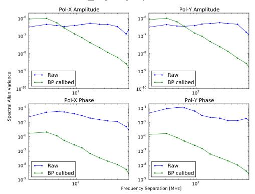
Figure 2: The spectral Allan variances (SAVs) of amplitude (top panel) and phase (bottom panel) as a function of frequency separation. Median values of the SAVs among 27 antennas are plotted.
