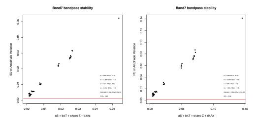
(a) SD (left) and PE (right) of bandpass amplitude variation at Band 7
