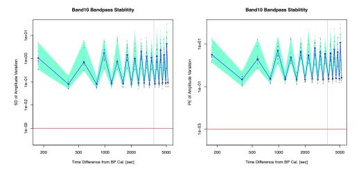
(a) SD (left) and PE (right) of bandpass amplitude variation at band 10.
