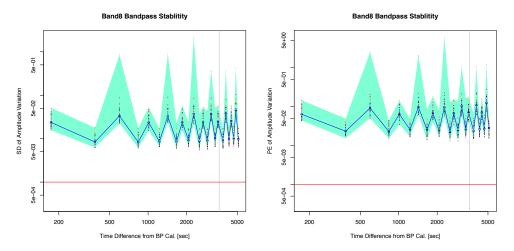
(a) SD (left) and PE (right) of bandpass amplitude variation at band 8.
