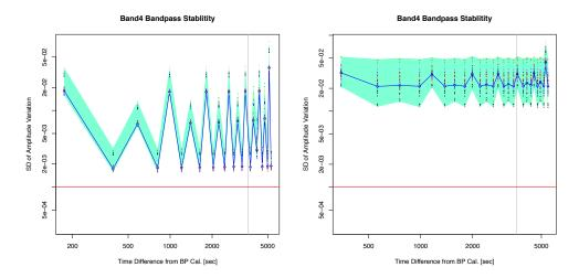
Figure 19: Time series of bandpass variation at band 4. Left and right panels stand for bandpass tables determined using FDM and TDM SPWs, respectively. See figure 4 caption for the legend.
