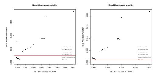
(a) SD (left) and PE (right) of bandpass amplitude variation at Band  $4\,$
