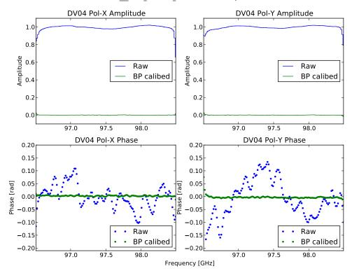
Figure 1: Cross power spectra of DV04 at Band-3. Top and bottom panels show the amplitudes and phases. Left and right panels stand for X and Y polarizations. Blue and green colors indicate the cross power spectra before and after bandpass calibration, respectively. The mean values of amplitude and phase are scaled to be unity and zero, respectively.
