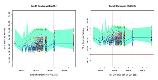
(a) SD (left) and PE (right) of bandpass amplitude variation at band 3 as a function of time difference between bandpass-calibration scans.
