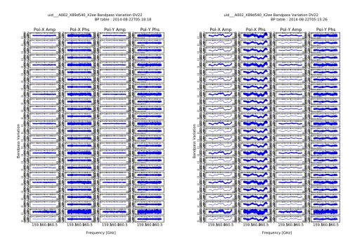
Figure 18: Comparison between FDM-FDM and TDM-FDM bandpass transfer. Bandpass variations at band 4 are plotted. (Left): Bandpass table was determined using the same FDM SPW. (Right): Bandpass table was produced in the TDM SPW and interpolated for FDM spectral channels.
