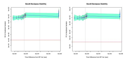
(a) SD (left) and PE (right) of bandpass amplitude variation at band 9.
