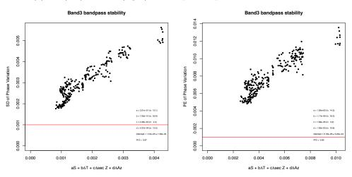
Figure 21: Predicted and measured bandpass variations in Band 3. The red horizontal line indicates the required stability of  $-30~\mathrm{dB}$ .
