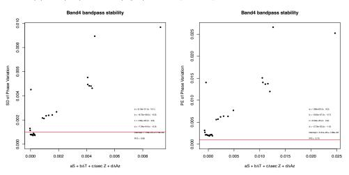
Figure 22: Predicted and measured bandpass variations in Band  $4\,$
