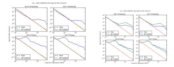
Figure 20: Spectral Allan variances of bandpass shape. Green and blue lines stand for the SAV before and after bandpass calibration, respectively. (Left): BP table was generated using the same FDM SPW. (Right): BP table was generated using the TDM SPW that covers the bandwidth of the target FDM SPW.
