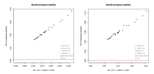
(a) SD (left) and PE (right) of bandpass amplitude variation at Band 9  $\,$
