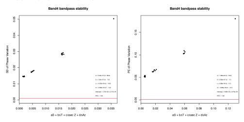
Figure 23: Predicted and measured bandpass variations in Band 4 FDM SPW
