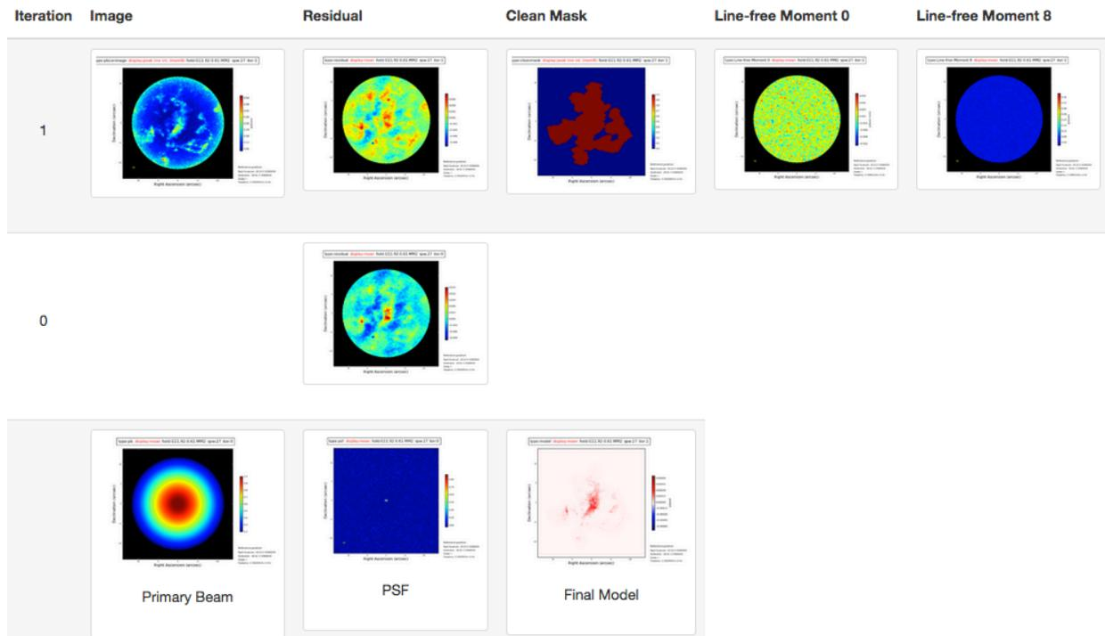
Figure 29: Example of an image cube details page including the line-free moment 0 and moment 8 images.
