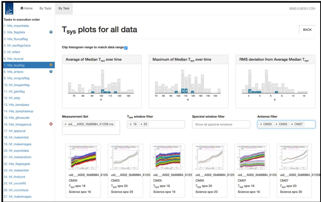
Figure 16: Same as Figure 15, but with a specific MS, Tsys window, and antenna filter set. The corresponding plots are displayed below, and their metric scores are shown by blue shading in the histogram plots.
