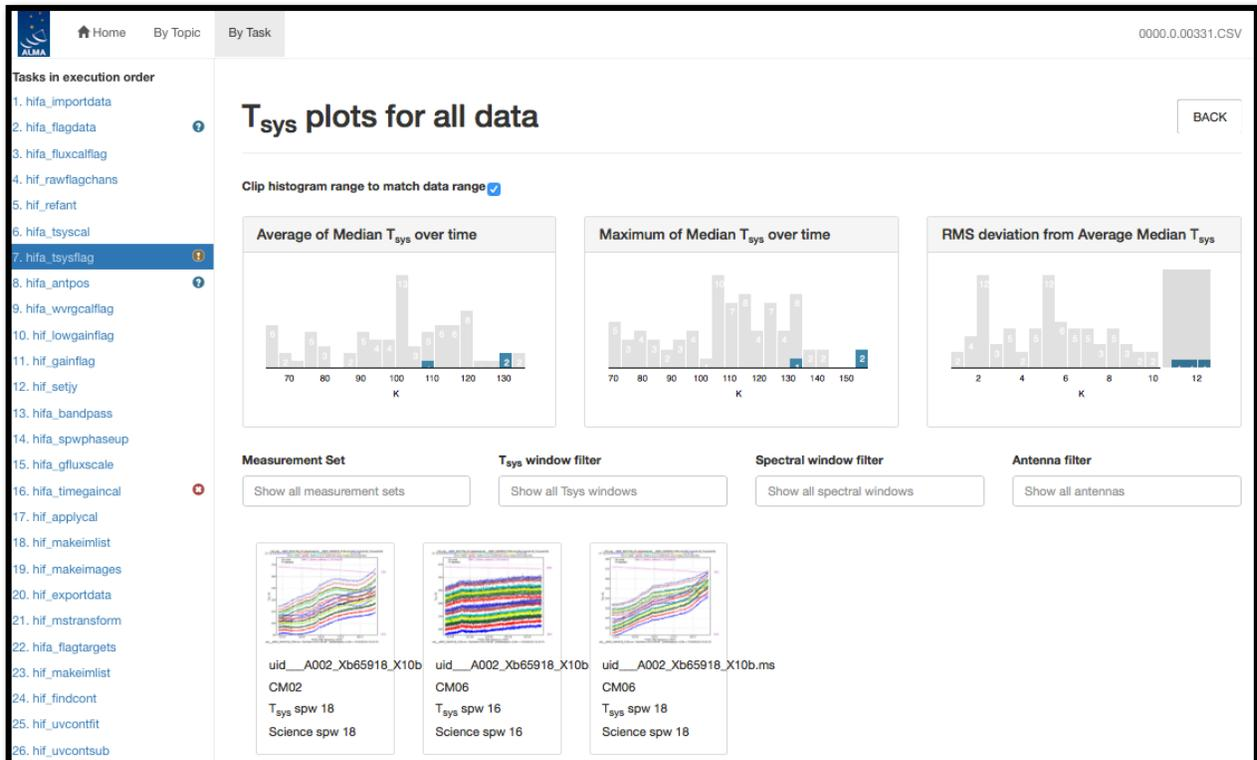
Figure 17: Same as Figure 15, but filtering to the plot of interest by using the mouse to draw a grey box on the highest histogram values in the RMS deviation from Average Median Tsys histogram plot (upper right). To clear the grey box filters on the histograms, click on any white space in the histograms.
