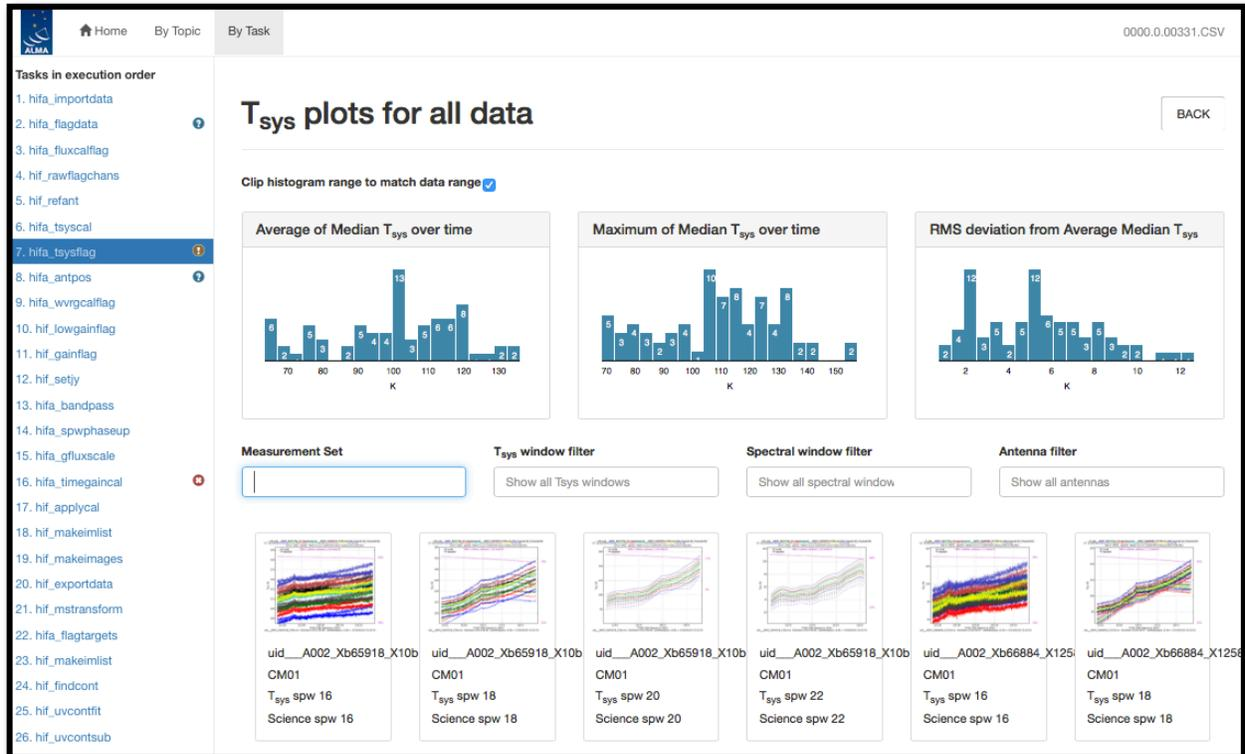
Figure 15: Unfiltered view of the hifa\_tsysflag sub-page. The page is arrived at by clicking on the measurement set link from the hifa\_tsysflag task page (Figure 13). Only the first row of plots are shown; many more appear below (one for each MS, antenna, spw combination). This page has histograms of three metric scores based on the median Tsys that can also be used to filter the plots that are displayed.
