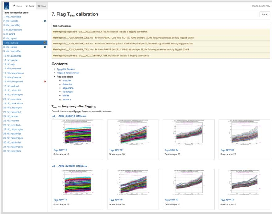
Figure 13: hifa\_tsysflag task page, showing the task notifications at the top, and diagnostic plots (Tsys for each spw grouped by MS). Further down on the page are flagging summary tables. To see the sub-page for this task, click on the measurement set name in blue above each set of plots. This will take you to a page of detailed plots for individual MS/antenna/spectral windows (see Figure 15 for an example).
