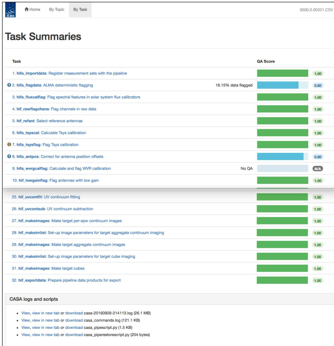
Figure 12: By Task summary view. The page has been truncated so both the top and bottom can be seen. Each pipeline stage is listed, along with its QA score (colored bars to the right), and links to the CASA logs and scripts.
