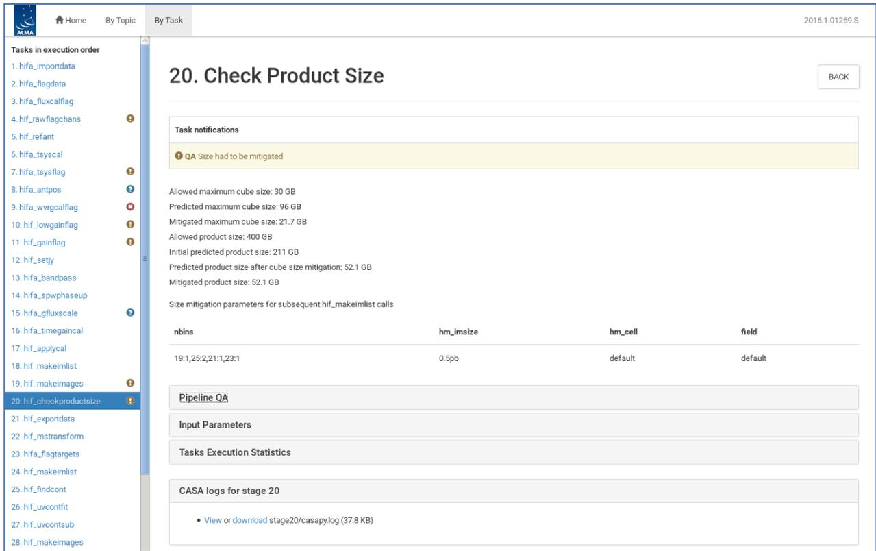
**Figure 24: Screenshot of new hif\_checkproductsize stage of IF Pipeline. In this example, the cubes for spw25 had to be binned by a factor of 2, and the FOV was limited to the 0.5 response point of the primary beam in order to get the products below the default thresholds. Before the mitigation the maximum cube would have been 96GB; after the mitigation, it is predicted to be 21.7 GB.**
