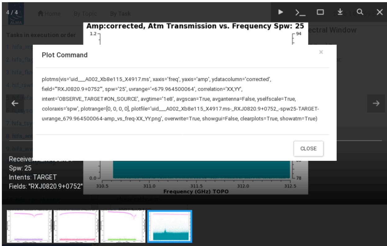
Figure 8: Example of WebLog plot with a "Plot command" link (>\_) that provides the CASA command for reproducing the plot.
